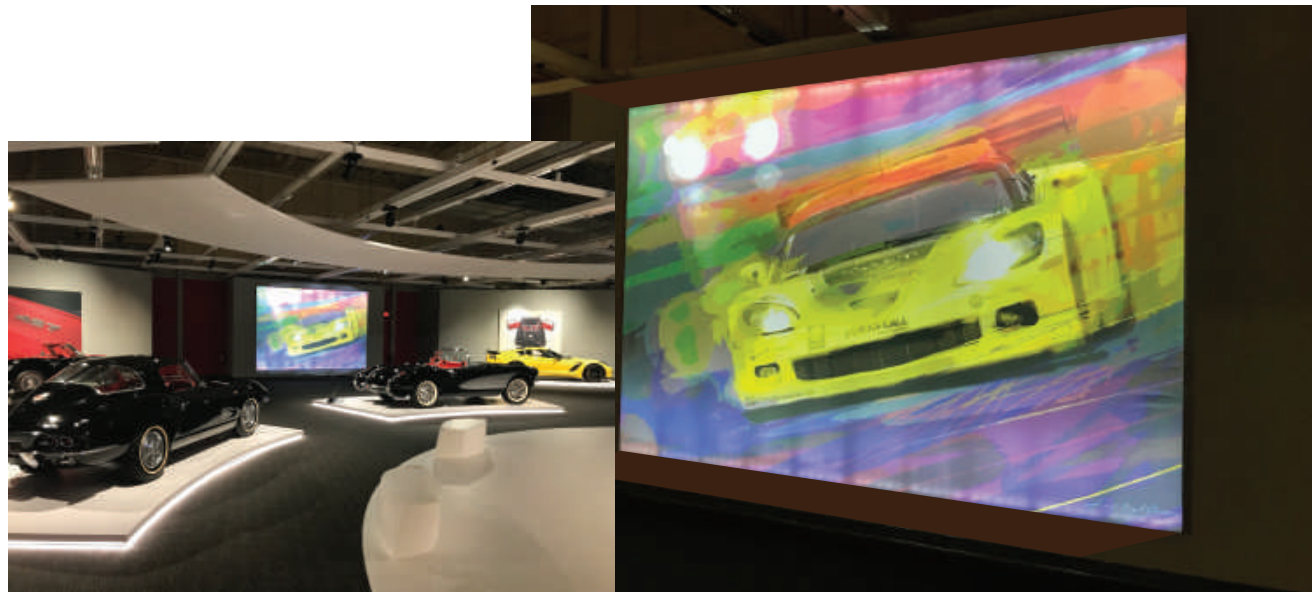
10' X 15' BACK LIT DIE SUB PRINTED FABRIC / MOUNTED IN ALUMINUM FRAME
